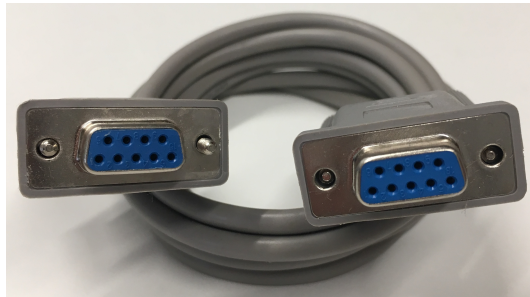
Fig. 2. A serial cable with 9-pin female connectors.
