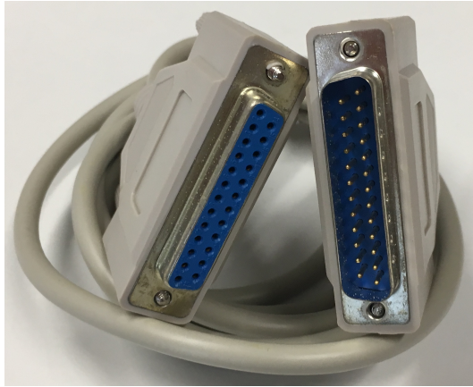
Fig. 1. A serial cable with 25-pin female (left) and male (right) connectors.
